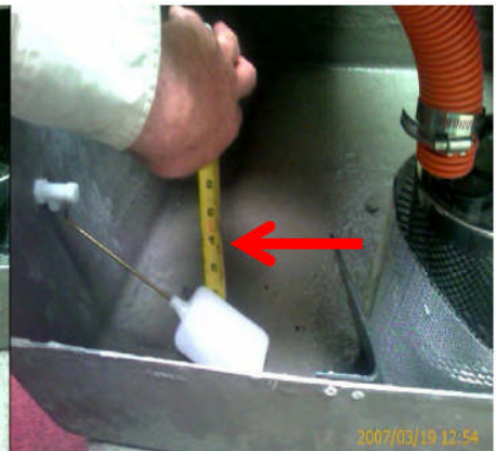
set water to 4 "deep then close unit up.
